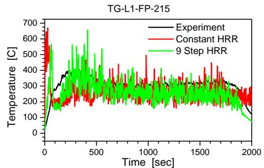
Figure 6. Gas temp in fire room at 2.15 m above fire source
