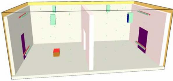
Figure 3 FDS 5 fire modeling for PRS\_D3 test facility
