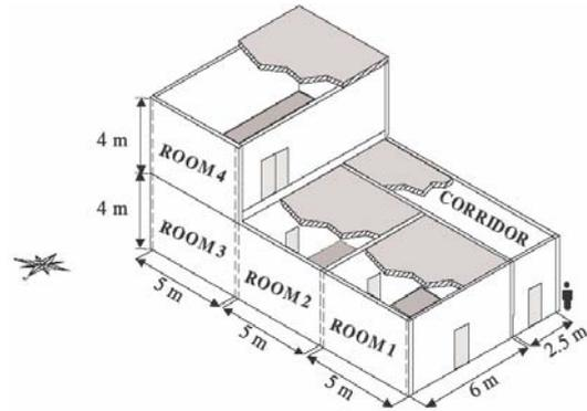
Figure 1 Perspective view of PRISME DIVA test facility
