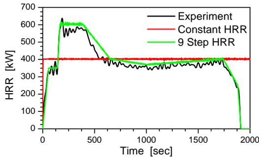
Figure 4 HRR profiles of PRS\_D3 test
