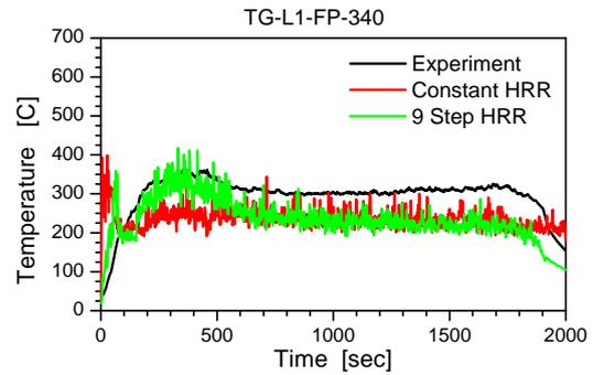
Figure 5. Gas temp in fire room at 3.4 m above fire source
