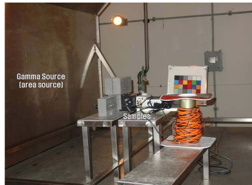
Fig. 3. A fiber optic communication system placed in the high dose-rate gamma irradiation facility.
