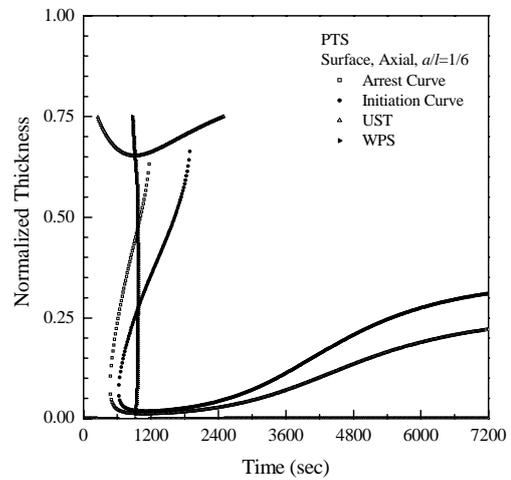
Fig. 2. Critical crack depth diagram for PTS
