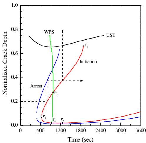
Fig. 1. Typical critical crack depth diagram
