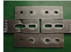
Photo 1. Fractured specimen 2SL2.5-1
