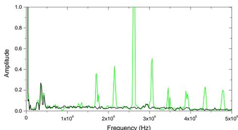
Figure 3 Signal Spectrums at the good bond and delaminated position
