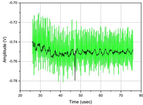
Figure 2 Typical zoomed waveforms at a good bond position (black line) and a delaminated position (gray line)
