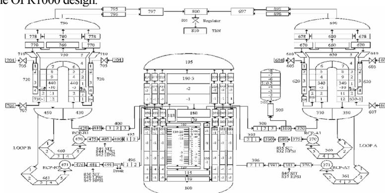
Figure 1 MARS Nodalization for Yonggwang 5 Load Reduction Test Simulation
