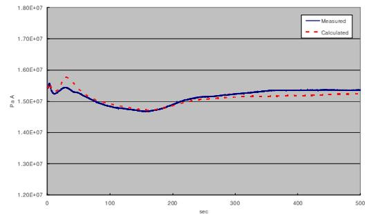
Figure 1 Comparison of Pressurizer Pressure Behaviors
