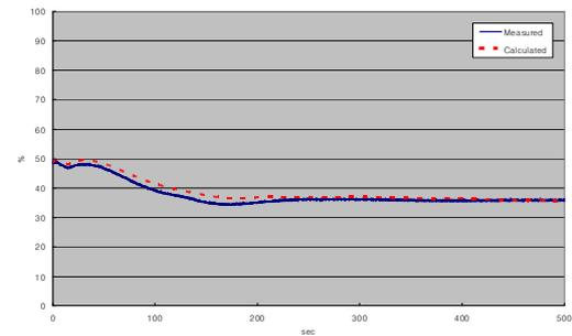
Figure 1 Comparison of Pressurizer Level Behaviors
