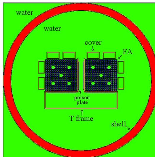
Figure 1. Nominal model of new fuel transport container
