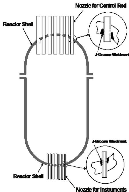
Figure 1. Schematic diagram of the penetration nozzles in a nuclear reactor vessel.
