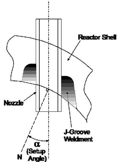
Figure 2. Definition of the nozzle setup angle ( $\alpha$ ) in a reactor vessel.
