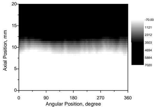
Figure 3. 3-dimensional distribution of the eddy current impedance from the specimen with a setup angle of 0 degree.
