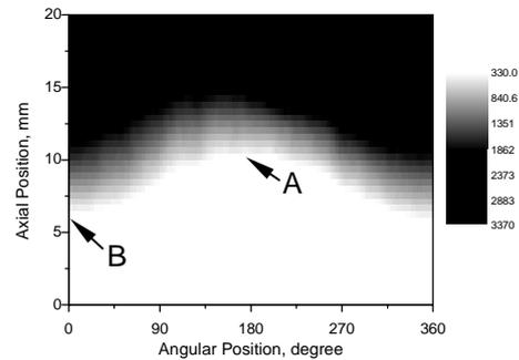
Figure 4. 3-dimensional distribution of the eddy current impedance from the specimen with a setup angle of 15 degrees.
