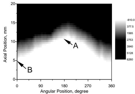
Figure 5. 3-dimensional distribution of eddy current impedance from the specimen with a setup angle of 21 degrees.
