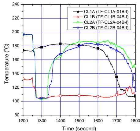
Figure 2 A variation of the fluid temperatures in the upper section of horizontal pipes of cold legs
