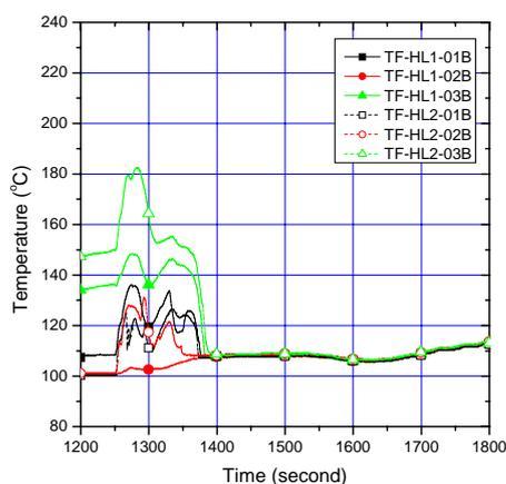
Figure 3 A variation of the fluid temperatures in the upper section of horizontal pipes of hot legs
