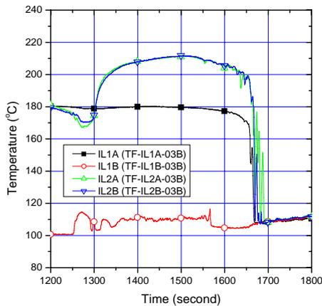
Figure 1 A variation of the fluid temperatures in the upper section of horizontal pipes of intermediate legs
