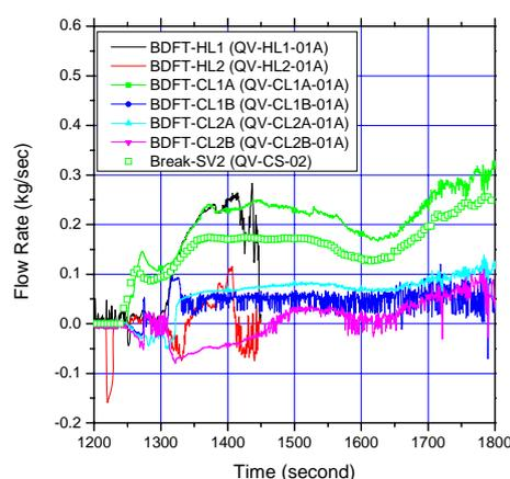
Figure 4 A variation of the steam flow rates in the RCS measured by using BiFlow flow meters
