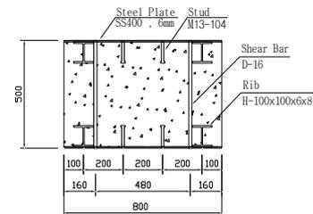
Fig 1. B-4R-2S400-4ST (1<sup>st</sup> and 2<sup>nd</sup>)
