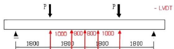
Fig 3. Loading Condition
