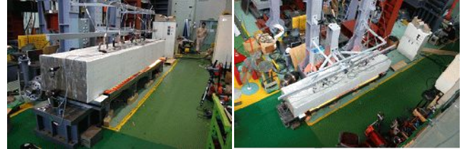
Figure 3. Specimen and Thermal Heat Panel
