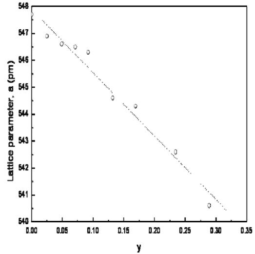
Fig. 4. Lattice parameter of  $(\text{U}_{1-y}\text{Gd}_y)\text{O}_2$  versus Gd content ( $y$ ) in  $(\text{U}_{1-y}\text{Gd}_y)\text{O}_2$  at a room temperature[1].
