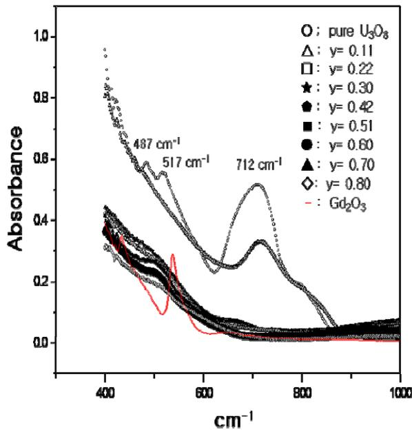
Fig. 3. FTIR spectra for the oxidized products of the Gd-doped  $\text{UO}_2$  [ $(\text{U}_{1-y}\text{Gd}_y)\text{O}_2$ ].
