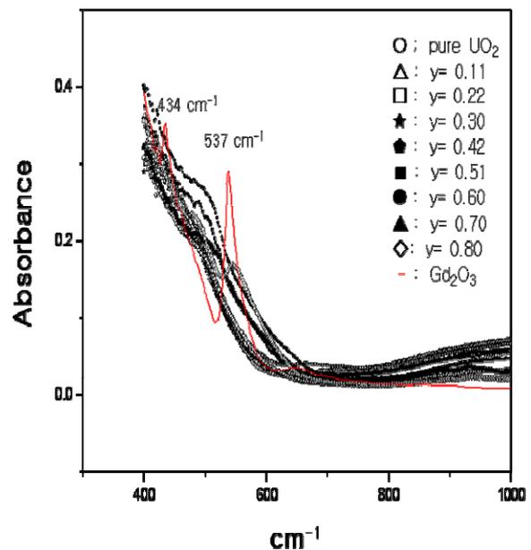
Fig. 2. FTIR spectra for the samples of Gd-doped  $\text{UO}_2$  [ $(\text{U}_{1-y}\text{Gd}_y)\text{O}_2$ ].
