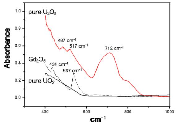
Fig. 1. FTIR spectra for the undoped  $\text{UO}_2$  and  $\text{U}_3\text{O}_8$ .
