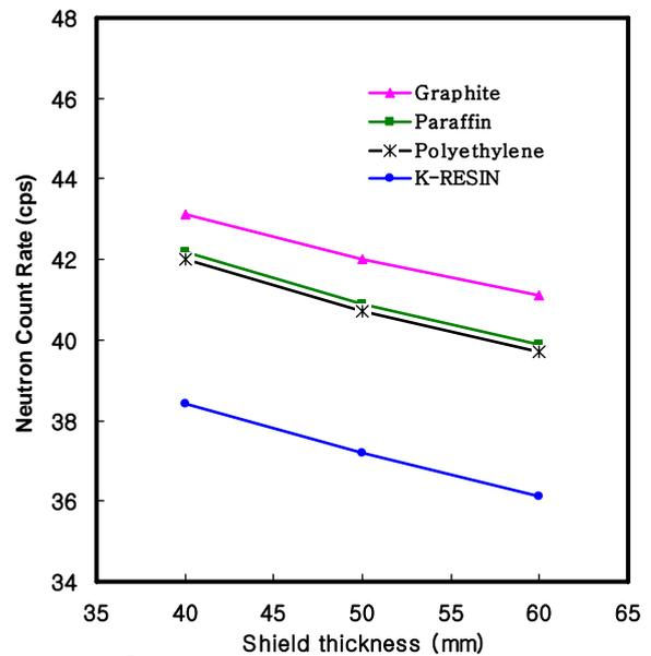
Fig. 2 Neutron count attenuation curve on shield materials and thickness
