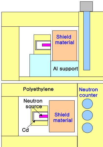
Fig. 1 Neutron shield test model
