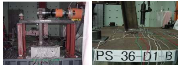
Figure 3. Specimen and Thermal Heat Panel
