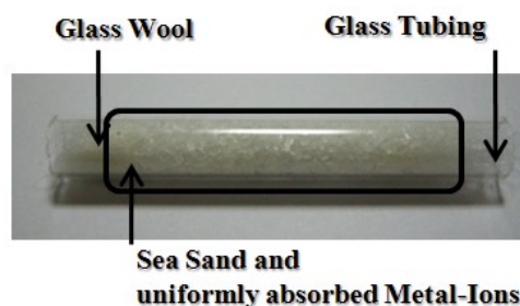
Fig. 2. Mock-up specimen in which the surface of the sea sand was impregnated with metal-ions
