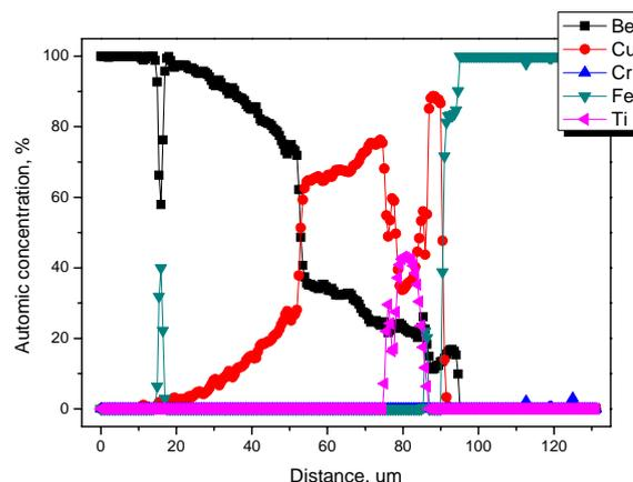
Fig. 2. Auger line profiles for the joint specimen with a Ti/Cu interlayer.
