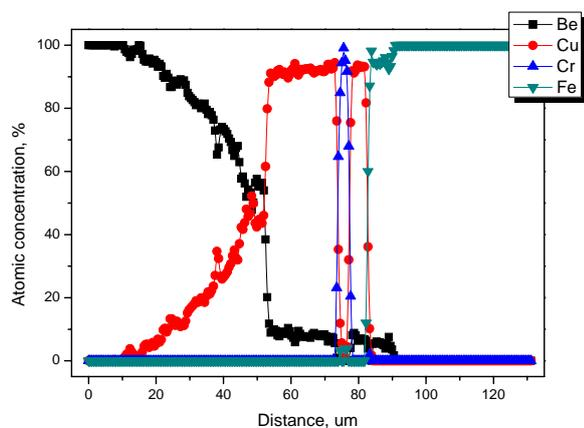
Fig. 1. Auger line profiles for the joint specimen with a Cr/Cu interlayer.
