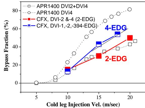
Fig. 2 Direct ECC bypass fraction
