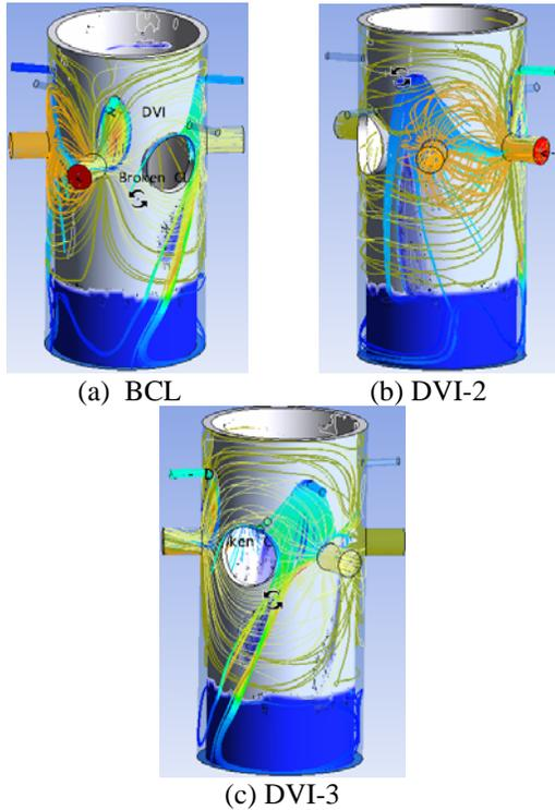
Fig. 1 CFX Simulation of Air-Water direct ECC bypass phenomena for  $V_{\text{coldleg,air velocity}}=18$  m/s ; (a) flow pattern at broken cold leg (DVI-4), (b) at DVI-1, (c) at DVI-3.
