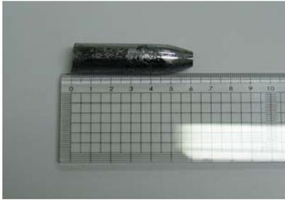
Fig. 2 CZT Crystal grown with the Bridgman method
