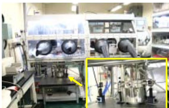
Fig. 1. Glove interfaced with reaction vessel and spectroscopic components.
