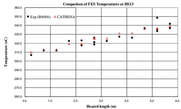
Fig. 2 Comparison of FES Temperatures between Test B9006 Data and CATHENA Results
