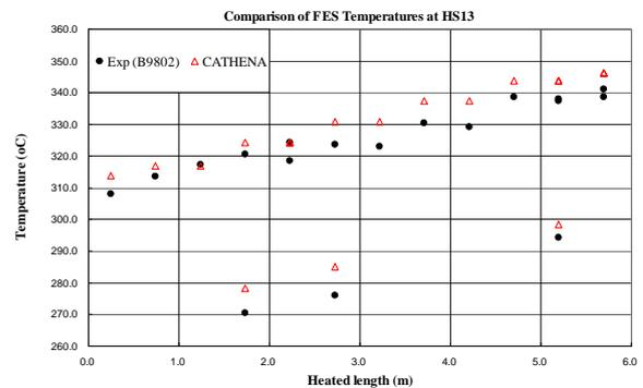
Fig. 3 Comparison of FES Temperatures between Test B9802 Data and CATHENA Results
