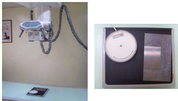
Figure 1. The figure of experimental system setup and arrangement of edge test device and ion chamber.
