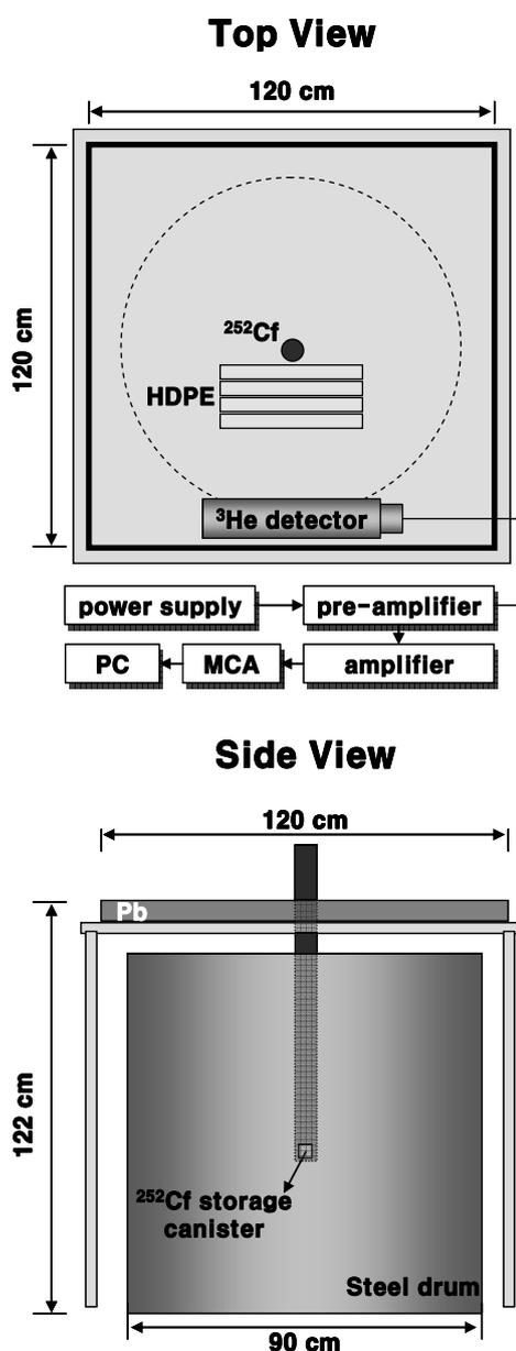
Fig. 1. Schematic Diagram of in-house developed neutron measurement system composed of source, detector, etc.
