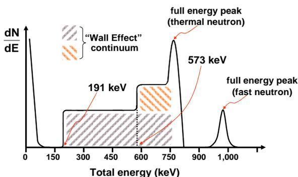
Fig. 2. A typical pulse-height spectrum from  $^3\text{He}$  proportional counter in which there is a “wall-effect”.
