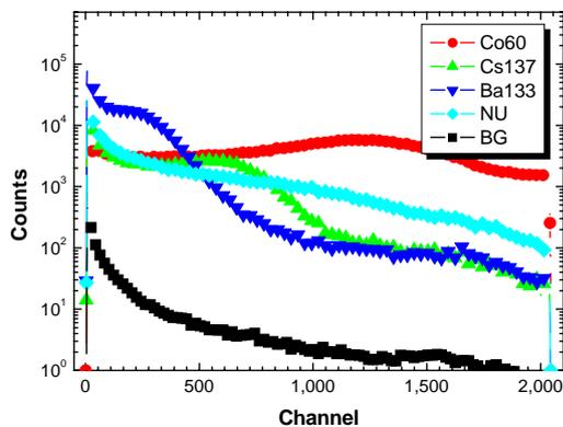
Fig. 3. Spectral distribution obtained with BC-412 plastic scintillator.
