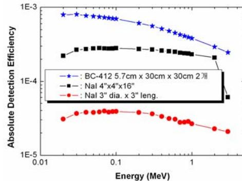
Fig. 1. Absolute detection efficiency of three different detectors
