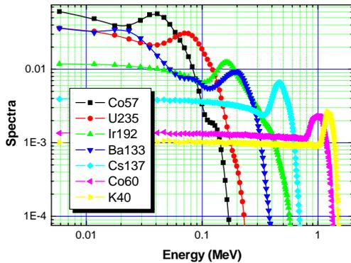
Fig. 2. Spectral distribution calculated by MCNPX
