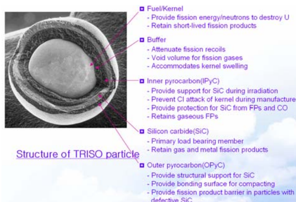
Fig.1. The structure of the TRISO particle.
