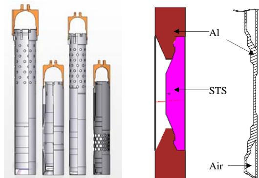
Fig. 1. Irradiation cans for 5, 6 and 8 inch crystals and enlarged neutron screens.
