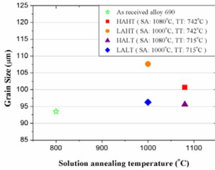
Fig. 3. Relation of between grain size and SA temperature.
