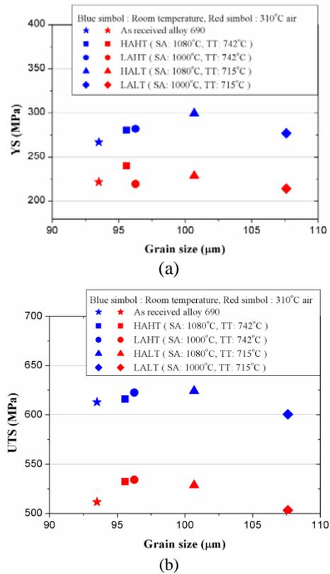
Fig. 4. Relation of between grain size and strength in two temperature conditions
