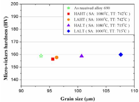
Fig. 5. Relation of between grain size and hardness in room temperature conditions
