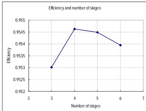
Fig. 2. Number of Stage Dependency for Efficiency
