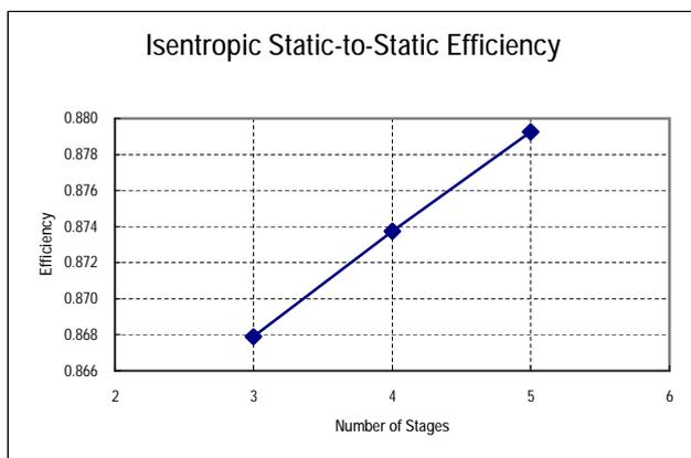
Fig. 3. Isentropic Static-to-static Efficiency
