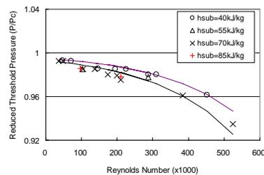
Fig. 3. CHF-TP for the Re and the inlet subcooling
