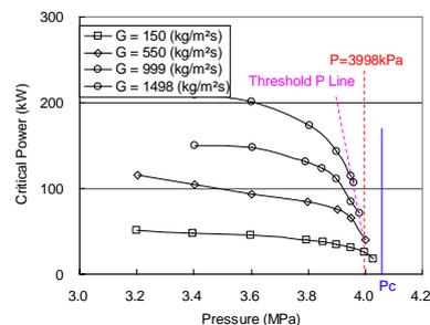
Fig. 1. Experimental evidence of the TP
