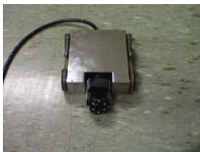
Figure 6. Upper head visual inspection robot.
