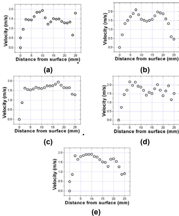
Fig. 4. Velocity distribution from the pebble surface center along the line a, b, c, d and e of Figure 2.
