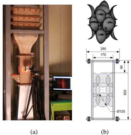
Fig. 1. Experiment system. Wind tunnel and PIV system(a), Test section geometry (b)
