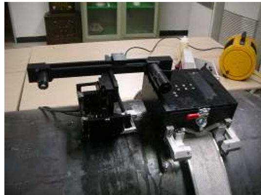
Fig 6. Modified DMW PA scanner
