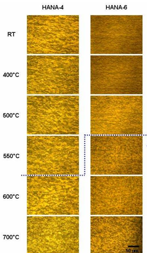
Fig. 1. Optical microstructures for HANA-4 and HANA-6 strips heat-treated various temperatures for 1 h.
