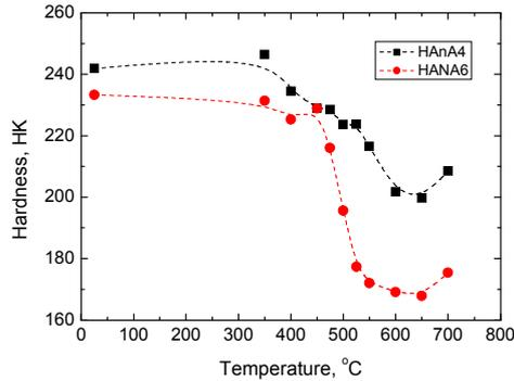
Fig. 2. Knoop Hardness number of HANA-4 and HANA-6 strips heat-treated various temperatures for 1 h.
