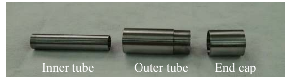
Fig 1. View of the fuel rod welding specimen components.
