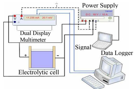
Fig. 1. The experimental equipments and system circuit.
