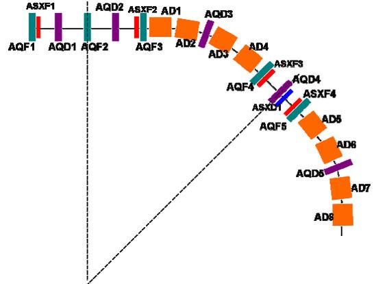
Fig. 1. Lattice layout and naming scheme in "A" super-period
