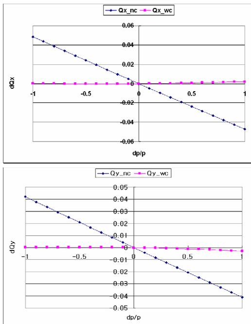
Fig. 3. Tune shift as a function of momentum spread for horizontal tune (upper figure) and vertical tune (lower figure).
