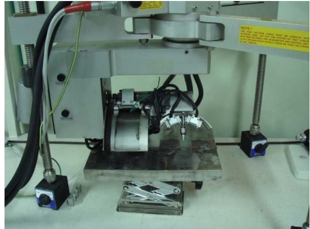
Fig. 1. Residual Stress Measurement Apparatus by Using X-ray Diffraction
