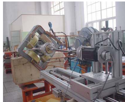
Fig 5. Prototype of PEFP quadrupole magnet.
