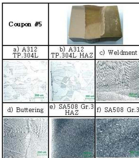
Fig. 3. Micro Structure of Coupon #5
