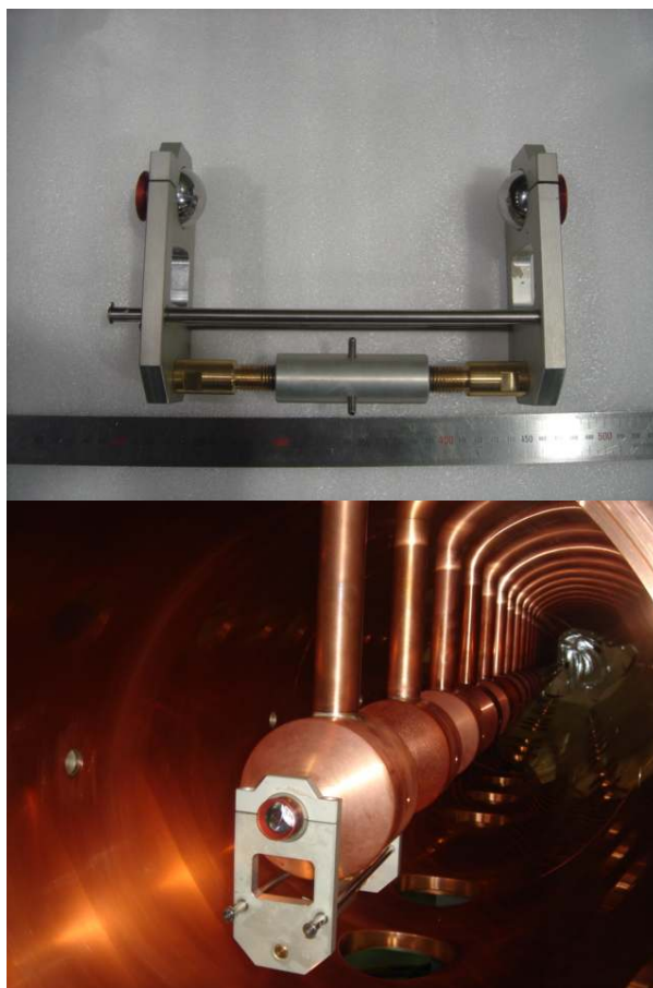
Fig. 2. Laser reflector holder for the drift tube alignment. The holder can fix two reflector which can be seen each laser tracker.
