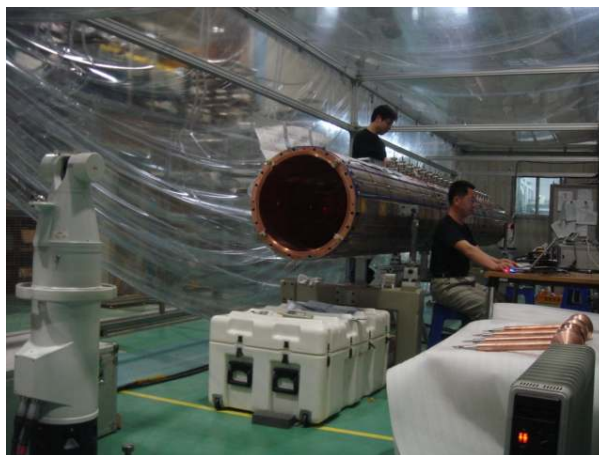
Fig. 1. Drift tube align procedure was accomplished with two laser trackers to real time position measurement. To improve the accuracy of laser tracker, all works are done in the vinyl house.
