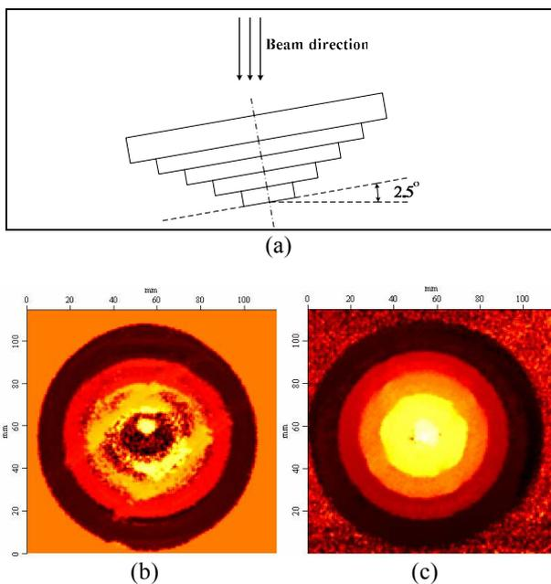
Figure 3. (a) Geometry of the test block. (b) C-scan image with the immersion sensor whose center frequency is 5 MHz. (c) C-scan image with waveguide sensor whose beam radiation angle is tuned.
