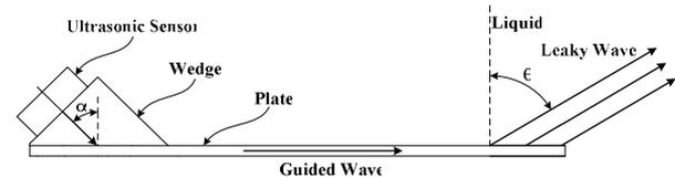
Figure 1. Generation of the guided wave and propagation of the leaky wave
