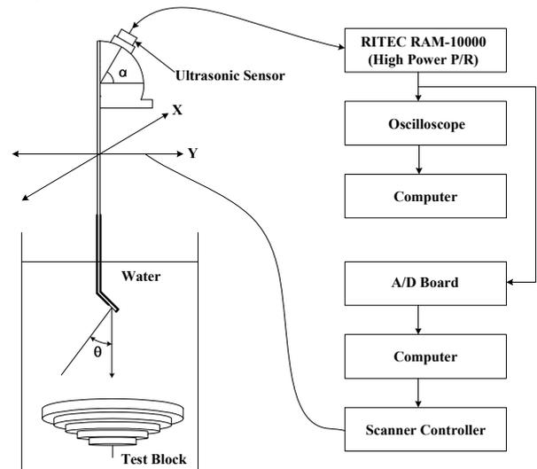
Figure 2. Experimental setup for the volumetric inspection by using waveguide sensor
