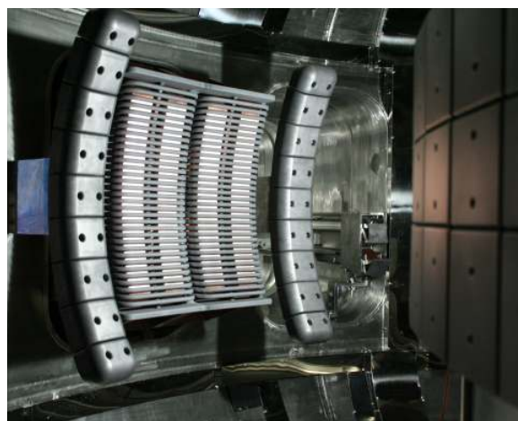
Fig. 1. The ICRF antenna has been installed in the KSTAR vacuum vessel in July 2007.
