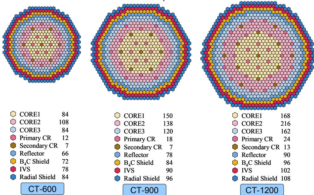
Fig. 1 Core Layout for the Variable-Cladding-Thickness Designs
