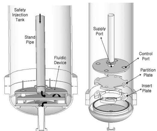
Fig. 1 Structure of APR1400 SIT.
