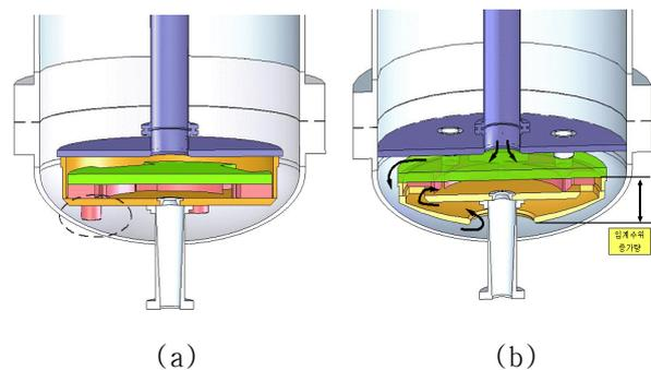
Fig. 2 SITs with modified control ports (a) and modified supply port (b).
