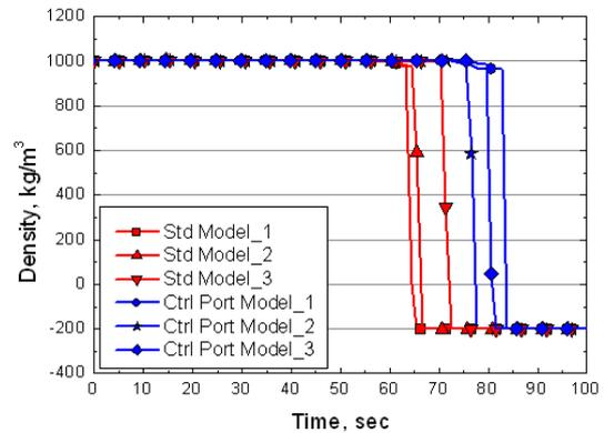
Fig. 5 Comparison of initiation time of air discharge
