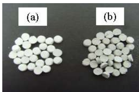
Fig. 1 Photograph of SA before(a) and after (b) heat treatment at 600°C.
