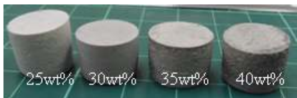
Fig. 3 Photograph of wasteform containing rare earth (Y, La, Ce and Nd) oxides
