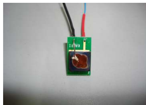
Fig. 1. The CZT detector fabricated in our work. The CZT crystal was grown with High Pressure Bridgman method.
