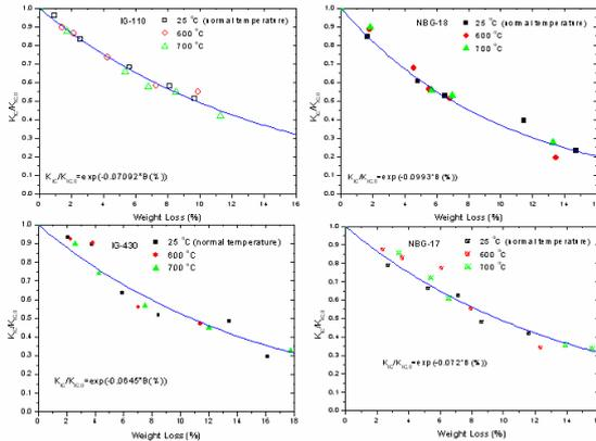
Fig. 2. Effect of weight loss on fracture toughness (IG-110, IG-430, NBG-18, and NBG-17)
