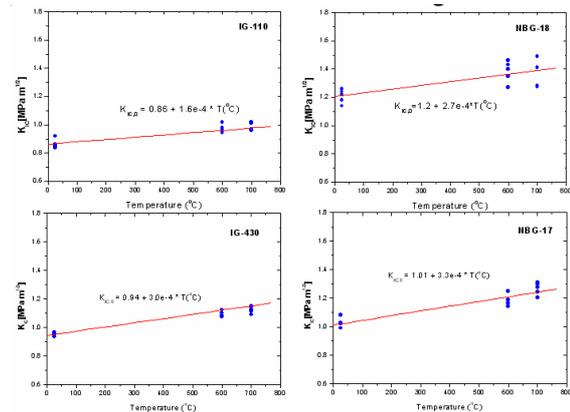
Fig. 1. Fracture toughness vs. temperature curves of nuclear graphite (IG-110, IG-430, NBG-18, and NBG-17)
