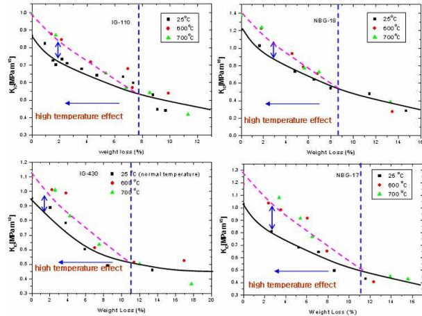
Fig. 3. Effect of high temperature effect on fracture toughness (IG-110, IG-430, NBG-18, and NBG-17)
