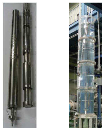
Fig. 2. Three double cladding fuel rod mockups and an outer tube(left)
