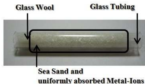
Fig. 1. Mock-up specimen; in which the surface of the sea sand was impregnated with metal-ions
