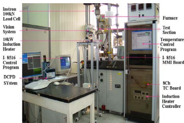
Fig. 1 A creep-fatigue crack test facility
